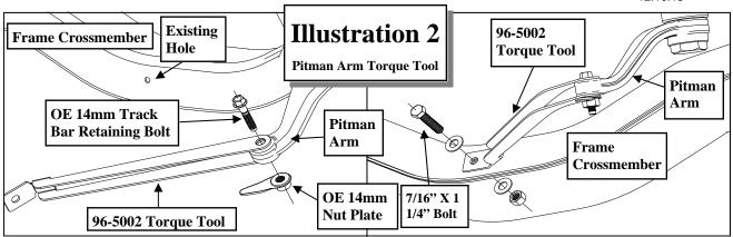
and hardware. See ILLUSTRATION 2. NOTE: The steering wheel may need to be turned in order for the hole in the torque tool and the frame crossmember to line up. Once the bolts are tightened the torque tool will align it's self properly.
